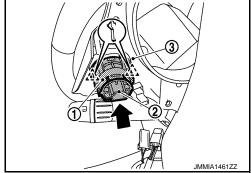
4. Disengage NATS antenna amp. fixing pawl and then remove NATS antenna amp. ② from push-button ignition switch ①.
